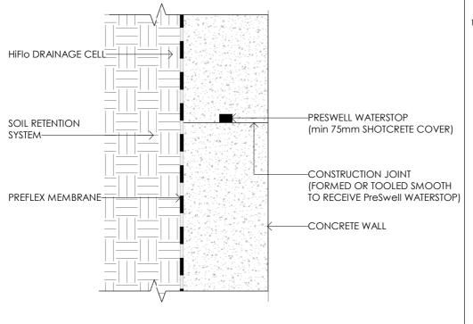
1. FORSPEC MAY REQUIRE AN ALTERNATE WATERSTOP BASED ON DESIGN CONDITIONS
